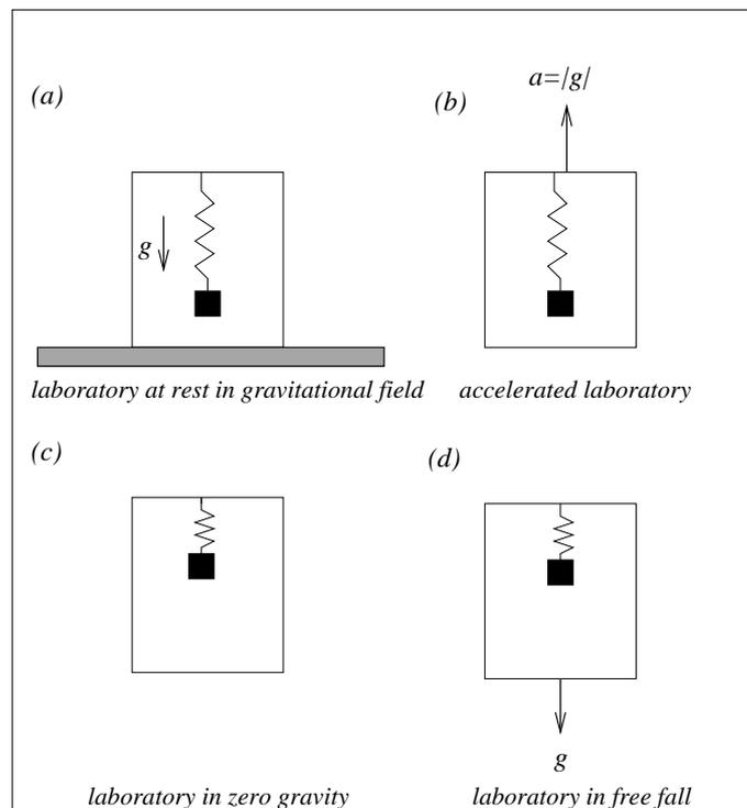
Figure 1: The Weak Equivalence Principle stipulates that the results of physics experiments in a gravitational field and in a laboratory accelerating at  $a = |g|$  are locally indistinguishable (panels (a) and (b)). The Strong Equivalence Principle asserts that the results of physics experiments in a region of zero gravity and in a laboratory in free fall in a gravitational field are locally indistinguishable (panels (c) and (d)).
