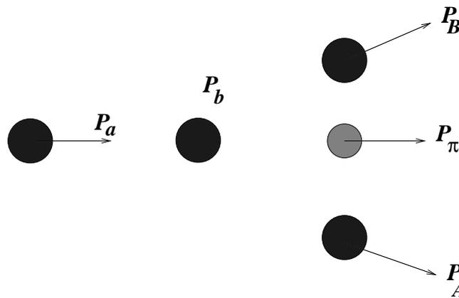
Figure 2: The collision between a moving proton and a stationary proton results in creation of a pion. The momentum-energy four vectors are  $\mathbf{P}_a$  and  $\mathbf{P}_b$  for the protons before collision,  $\mathbf{P}_A$  and  $\mathbf{P}_B$  for the protons after collision and  $\mathbf{P}_\pi$  for the pion.
