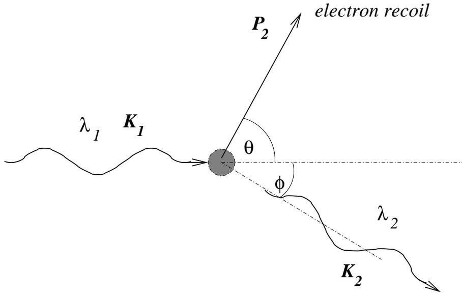
Figure 1: A photon of wavelength  $\lambda_1$  is scattered by an electron. The electron recoils and the photons is redshifted to wavelength  $\lambda_2$ .  $\mathbf{K}_1$  and  $\mathbf{K}_2$  are the momentum-energy four vectors of the photon before and after scattering, and  $\mathbf{P}_2$  is the momentum-energy four vector of the electron after scattering.
